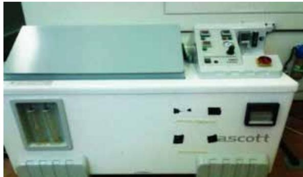
Fig 1. Salt Spray Chamber
